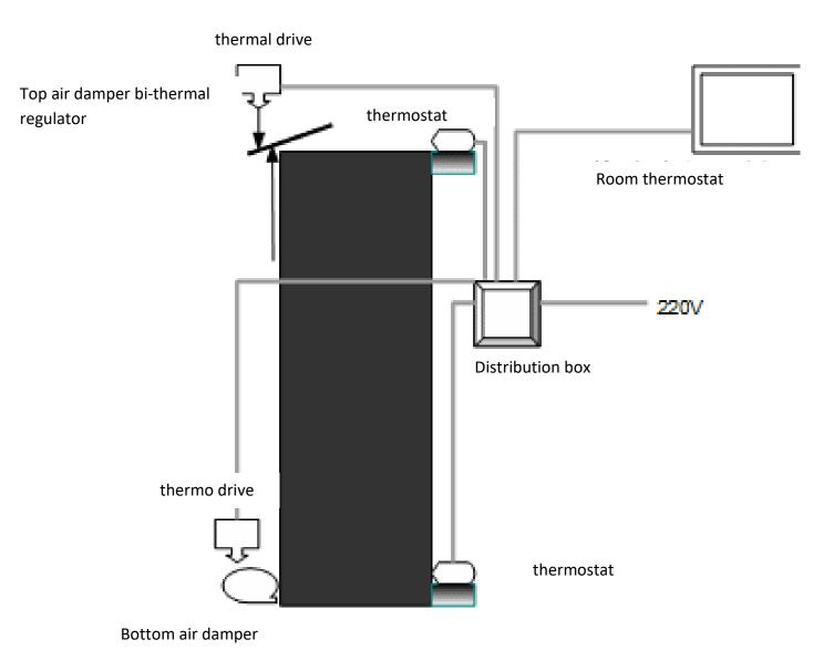
When using coal, peat briquettes, wood particles (chips), sometimes air needs to be delivered under the fuel load. This can be done by using ash grill and bottom air damper. Bottom air damper is operated with thermal drive, which is controlled by supply water flow thermostat.
